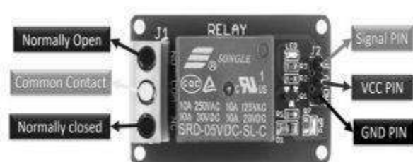
Fig 16 Relay Module Pin Diagram
